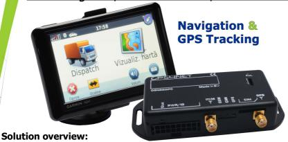
G4N01GAR is a bridge communication interface between the Garmin GPS navigation system and the GPS Tracker box which provides a direct interaction between the driver and dispatch center. The interface was designed to provide a two-way text messagery, transfer of routes and destinations and the tracking of status changing.
